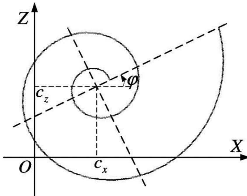
Fig. 1. Two turns of logarithmic spiral turned by the angle  $\varphi$  and shifted along the axis  $OX$  by the value  $c_x$  and along the axis  $OZ$  by the value  $c_z$  relative to the spiral origin
